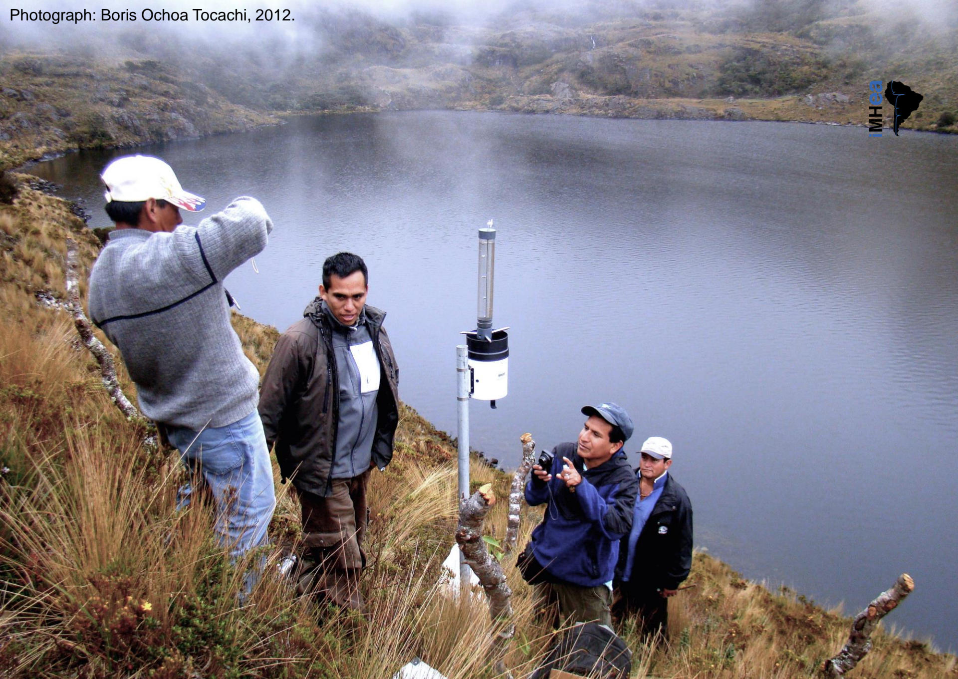
Precipitation: At least 2 tipping bucket rain gauges (res. 0.254 mm or better).
